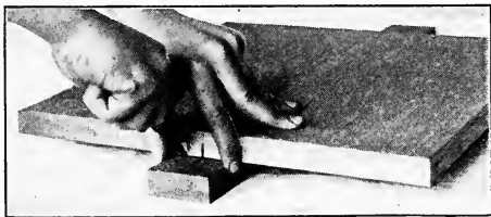
Fig. 321—Marking for Dowels
